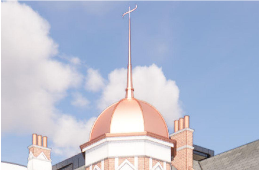
Figure 50: Perspective drawing extract of the proposed copper domed, segmented cupola with windvane / lightning rod to be reinstated in an interpretation of the original cupola
