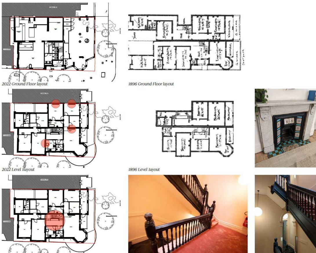
Figure 47: 2022 ground, level 1 and level 2 plan extracts with significant fabric circled in pink (left), 1896 plan extracts (middle) and photographs of the significant existing staircase and fireplace (right)
