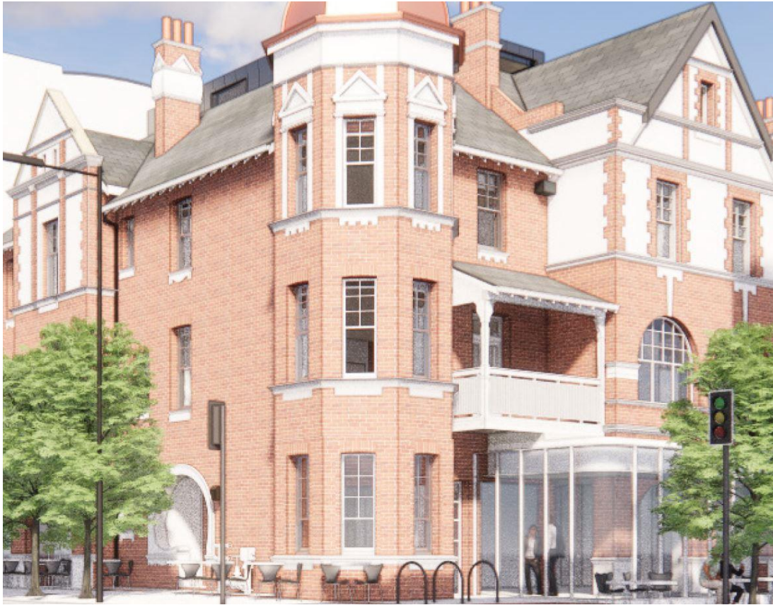
Figure 49: Perspective drawing extract of the proposed heritage slate roof, brick finish, render, and trims
